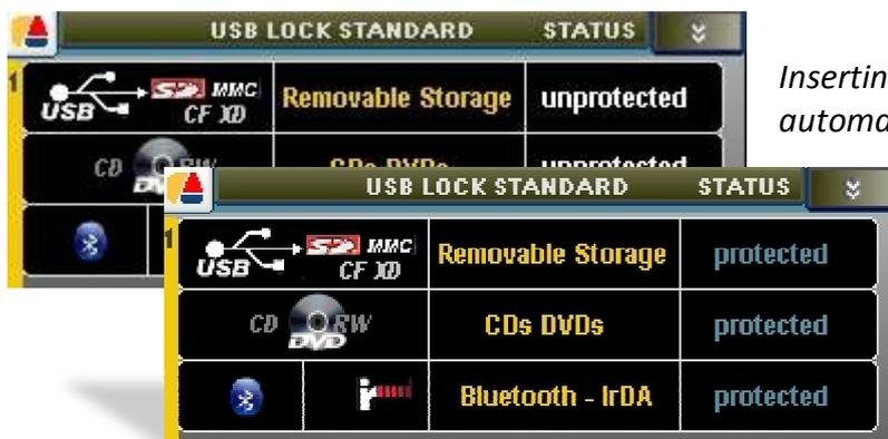
*Inserting the usb token unprotects all sectors automatically, allowing normal devices use.*
